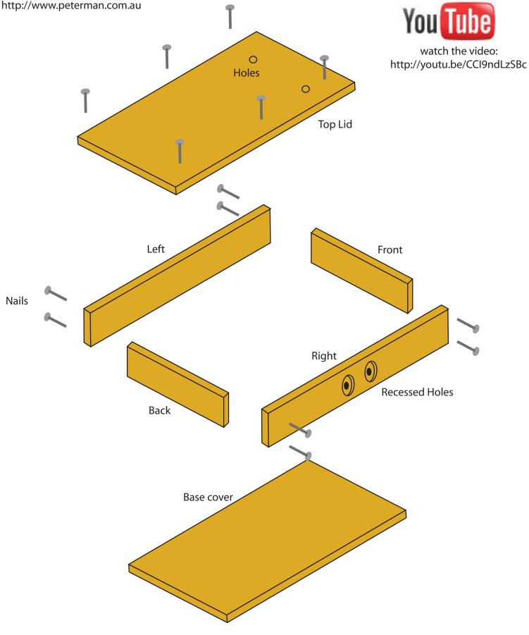
Top Lid 200x300mm x 12mm thick 2 holes 5mm diameter
